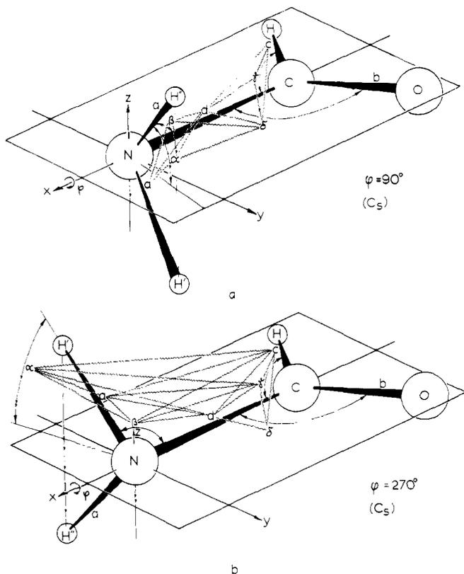
**Figure 1.** The definitions of the coordinate system, geometrical parameters optimized, and the couplings considered, for the saddle point  $\varphi = 90^\circ$  (a) and  $\varphi = 270^\circ$  (b) rotamers of formamide. In both cases the  $C_s$  symmetry has been assumed.
